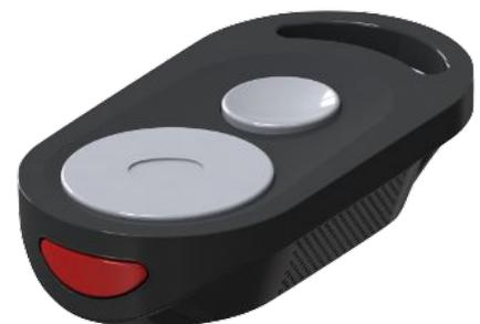
The “FN button #1” can for example be configured for “Queue” or “Repeat Message” functionality.
